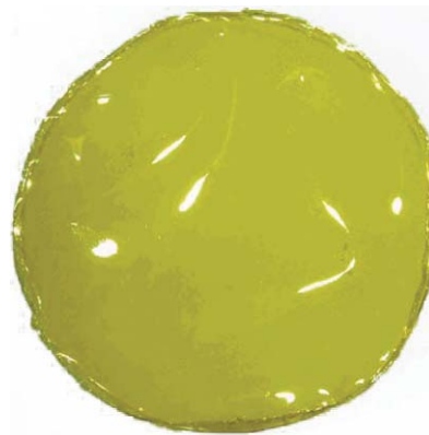
Fig. 4 A self-standing film of PIM-1 cast from a solution of THF.
